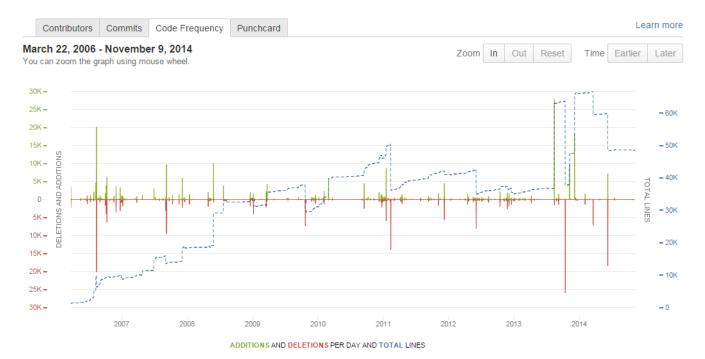
The green and red graphs with the left-hand scale show added and deleted lines of code per week respectively. The dotted blue line with the right-hand scale represents the total number of existing lines. The graph covers the whole project from its start to the current week.
